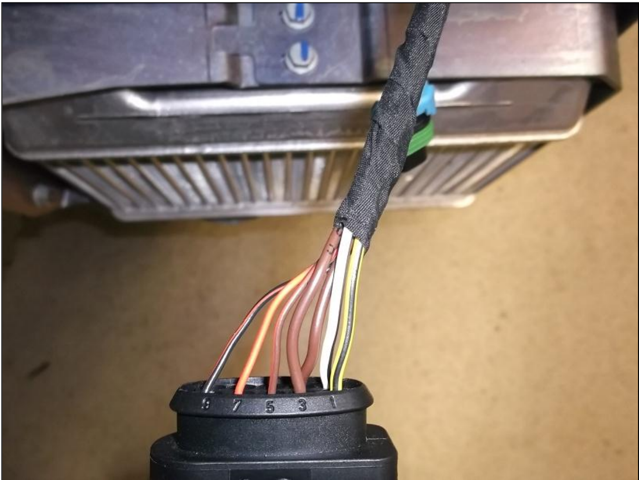
Bild 5: Original MB Stecker Figure 5: Original MB connector
